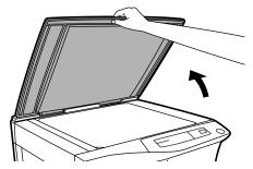
Place the original face down on the original table. Align it with the original scale and the centering (**>**) mark.
